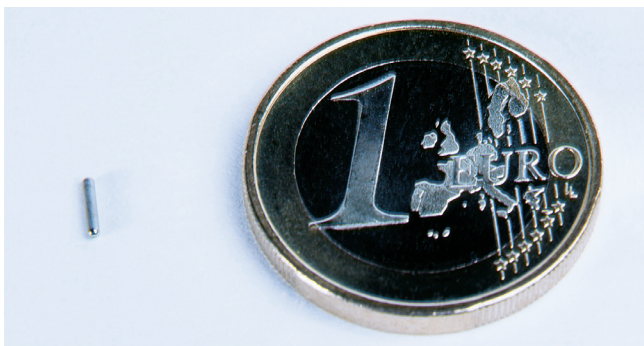
An Iodine-125 seed has a length of 4.5 mm and a diameter of 0.8 mm
